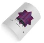
Step 2: Foil feeding and application on preprinted substrate via LED UV rays. Peeling off substrate film reveals metallization.
